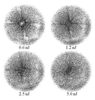
Fig. 2. The field evaporation image of tungsten at different laser power.
