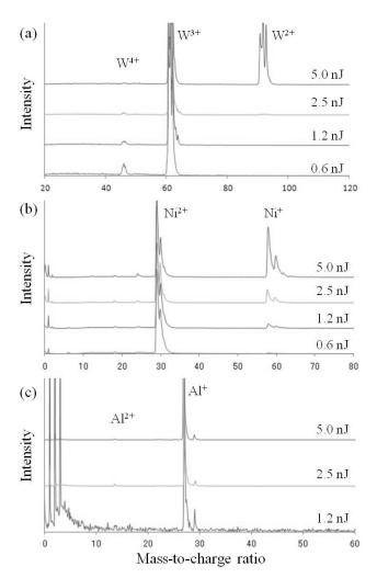
Fig. 1. The mass spectra of tungsten (a), nickel (b) and aluminum (c) with different laser power.
