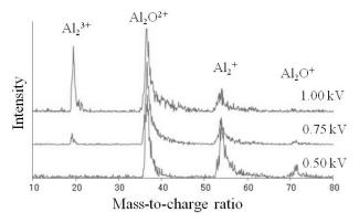
Fig. 3. The spectra of aluminum measured at different voltage pulse (standing voltage is 1.5 kV).
